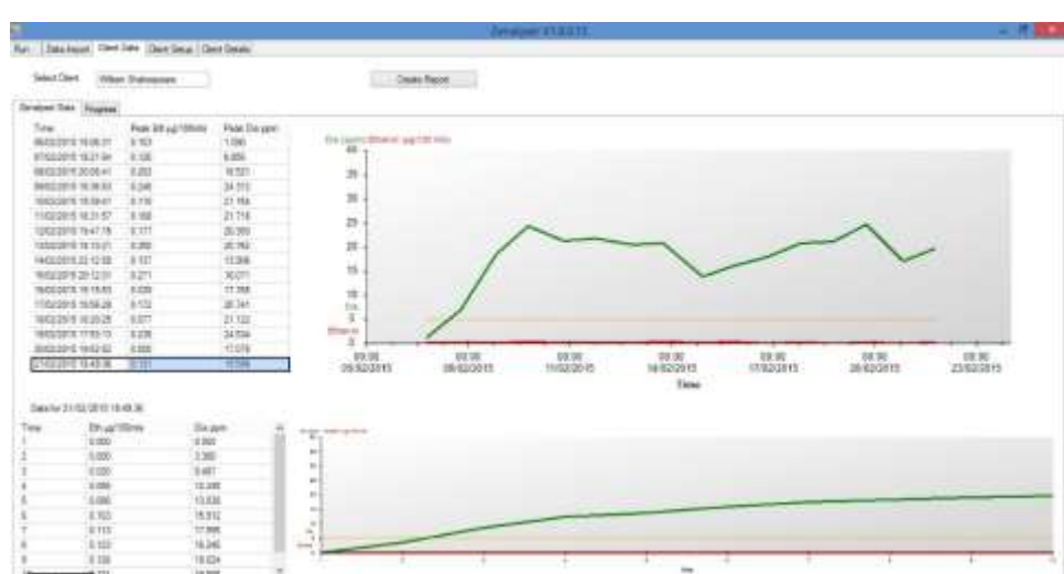
Fig. 1 Example of daily data sent from the Zenalyser ® - upper table and graph is cumulative data, lower table and graph is data of a single selected day's breath sample, second by second.
